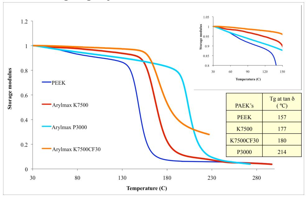
Measurements made on annealed samples using 3 point bend fixture (except Arylmax K7500CF30 measured (annealed) using single cantilever fixture)
