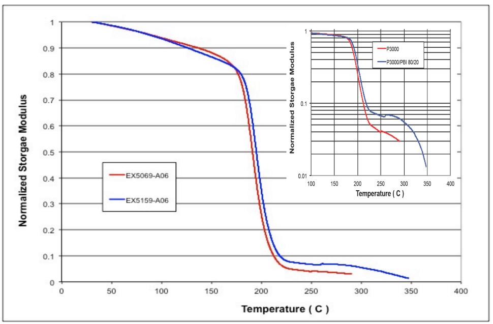
Measured on annealed samples using single cantilever.
