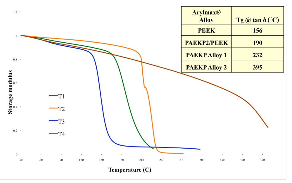
Measured on annealed samples using single cantilever.
