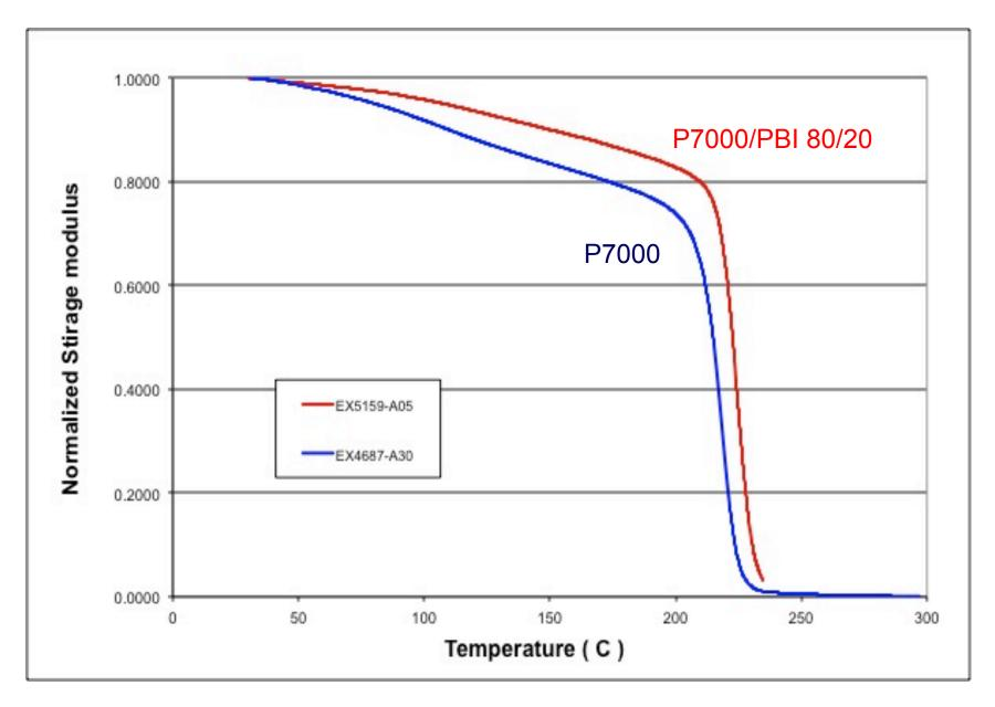
Measured on annealed samples using single cantilever.
