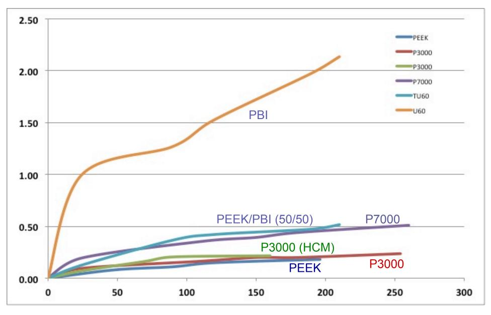
• Average of three Specimen immersed in 40% Sulfuric acid; Dimensions and Hardness was also checked.
