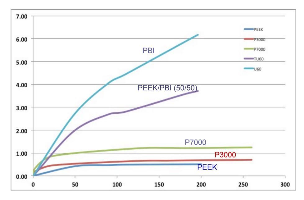
Average of three Specimen immersed in Water @ 60 °C; Dimensions and Hardness was also checked.
