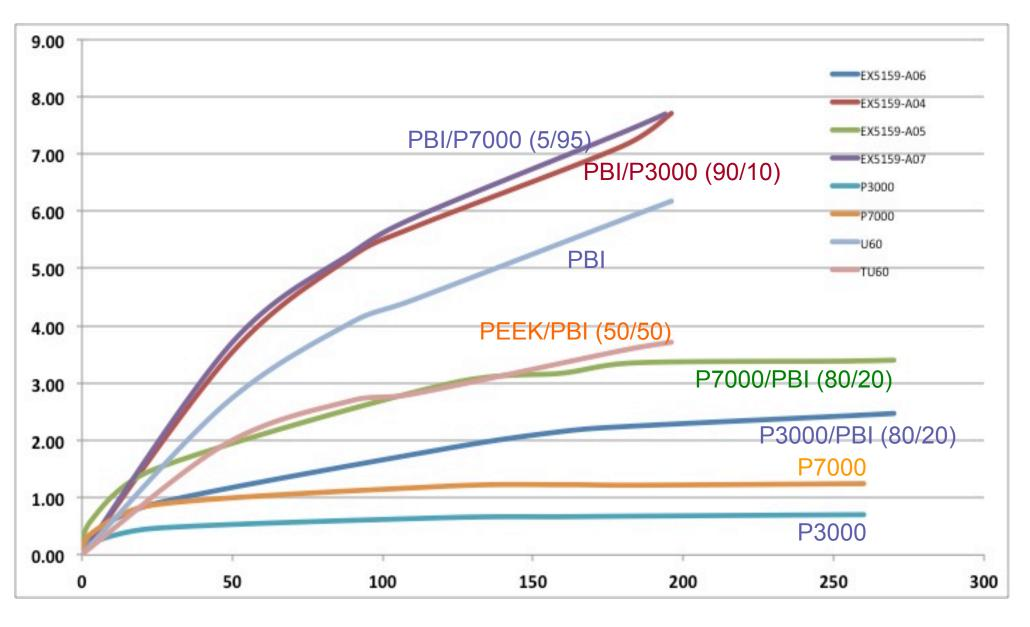
Average of three Specimen immersed in Water @ 60 °C; Dimensions and Hardness was also checked.
